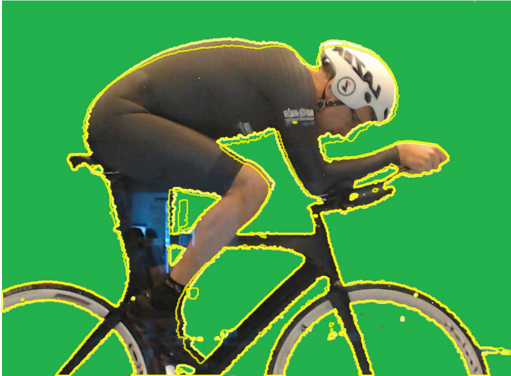
Figure 3 – Higher extension angle with Lazer Victor helmet (run 8 – figure) and aero shrug position (run 9 – contour).
