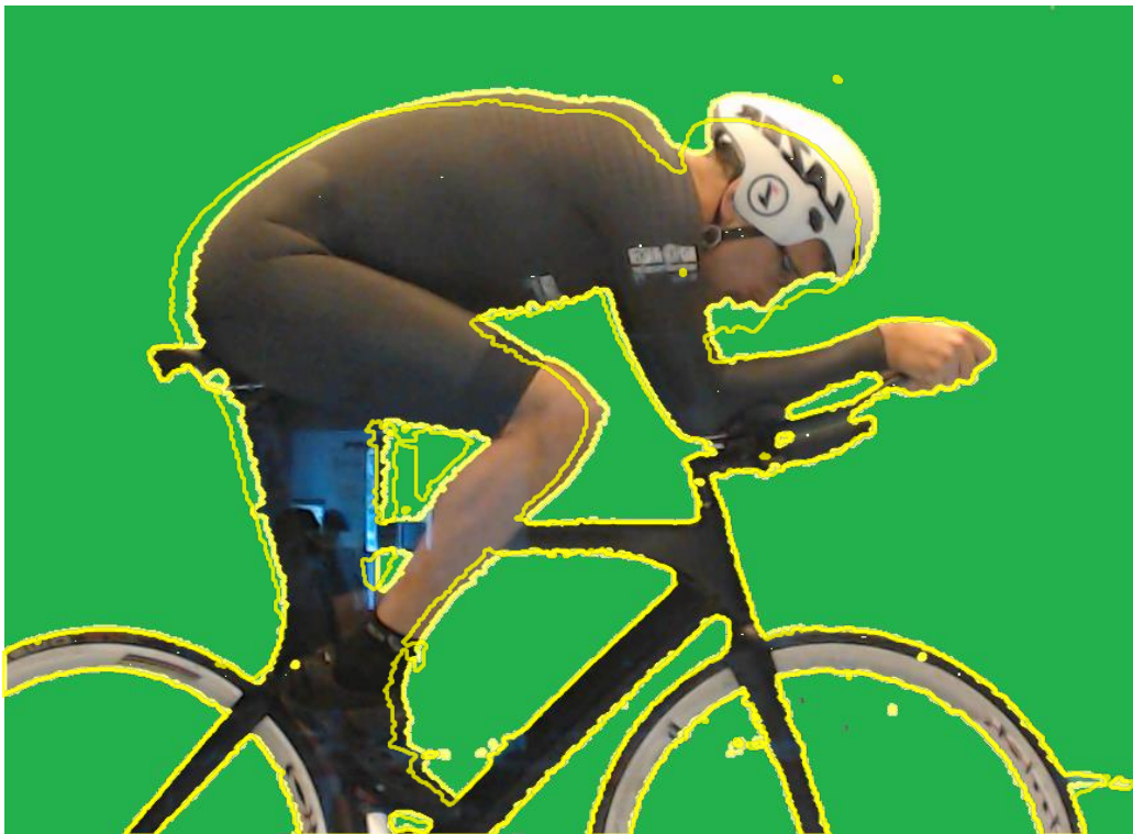
Figure 4 - Higher extension angle (run 8 – figure) and position further back on the saddle (run 10 – contour).
